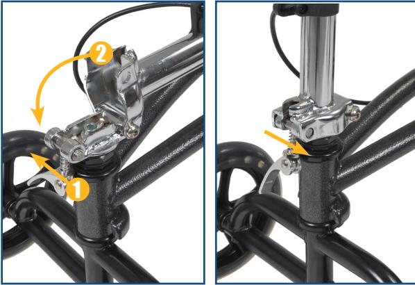
3. Slide locking mechanism into groove on tiller, depress locking handle to secure tiller lock.
